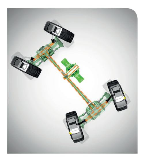
Maximum synergy is achieved with a new transmission that combines Merlo's experience in the field of hydrostatic transmissions with new technical solutions that afford the same performance, consumption and productivity as a conventional Continuously Variable Transmission. This system, designated Merlo CVTronic, is comprised of two hydrostatic motors with axial pistons and variable displacements that are supplied with oil by a load sensing hydrostatic pump driven directly from the diesel engine.
