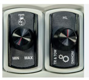
The EPD system also provides three manual operating modes: Transport and Tow, aimed at attaining or maintaining the desired speed with minimum fuel consumption; Heavy Load, used to obtain maximum performance during particularly demanding work such as excavation or snow clearance; and Inching mode.
