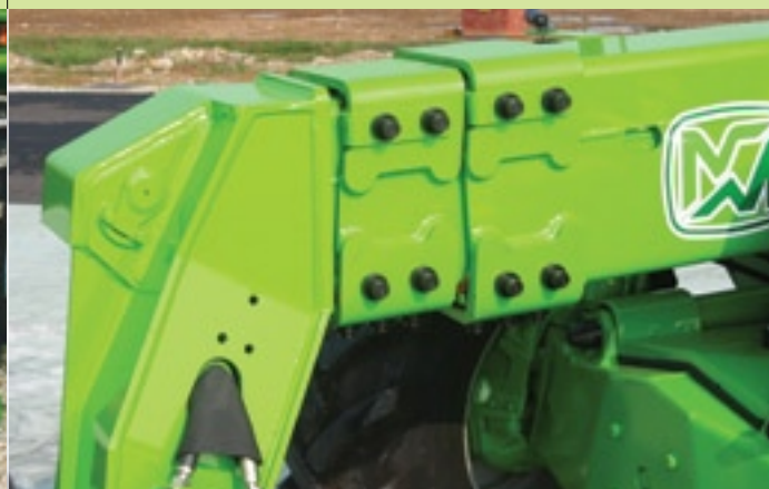
Boom sections slide on adjustable low-friction pads.
