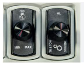
The EPD system provides manual control of several parameters such as Transport & Tow aimed at achieving or maintaining the desired speed with minimum energy consumption, Heavy Load for maximum performance during special processes such as excavation or removal of snow and Inching.
